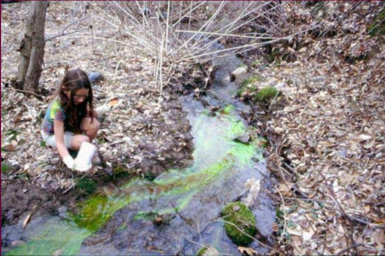
Fluorescein dye is introduced upstream of a western Virginia swallet.
