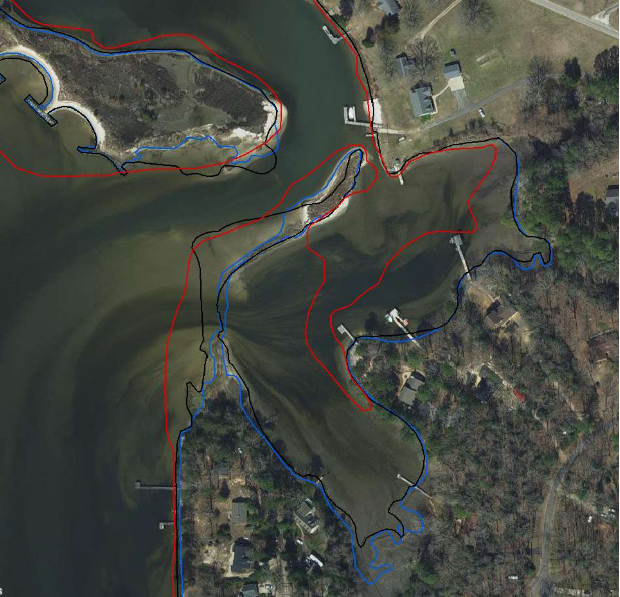
Figure 12 – 1937 shoreline (red), 2009 shoreline (black), and 2017 shoreline (blue) are depicted atop aerial site imagery taken from 2021. The spit on the eastern side of the mouth of Aberdeen Creek was expansive in 1937, had narrowed considerably by 2009, nearly breached by 2017, and was entirely compromised and breached by 2021. The one remaining island remnant of the spit present in 2021 has since completely disappeared, leaving the entire mouth of the creek unprotected from flooding impacts.
