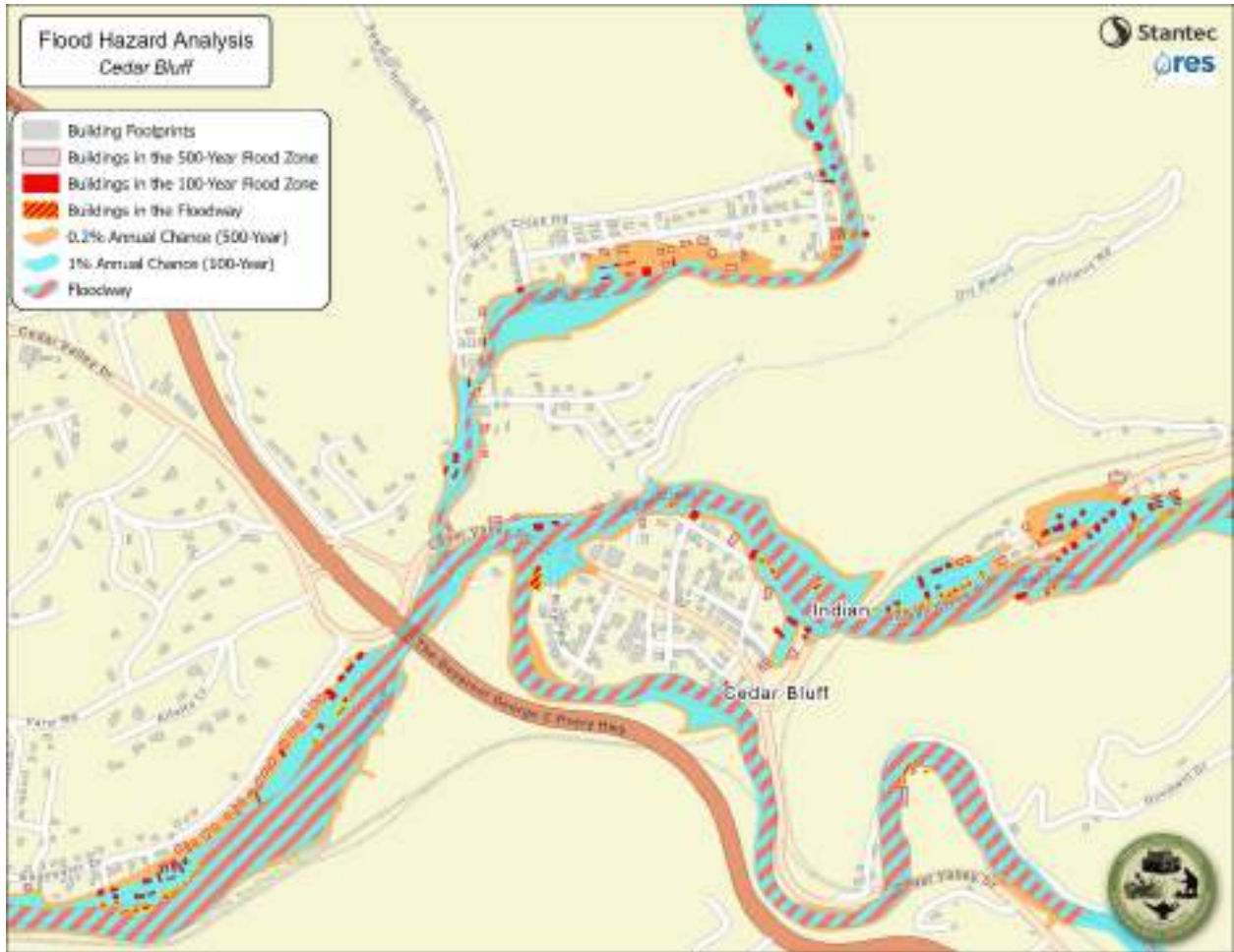
Figure 633: Flood Hazard Analysis – Cedar Bluff Area
