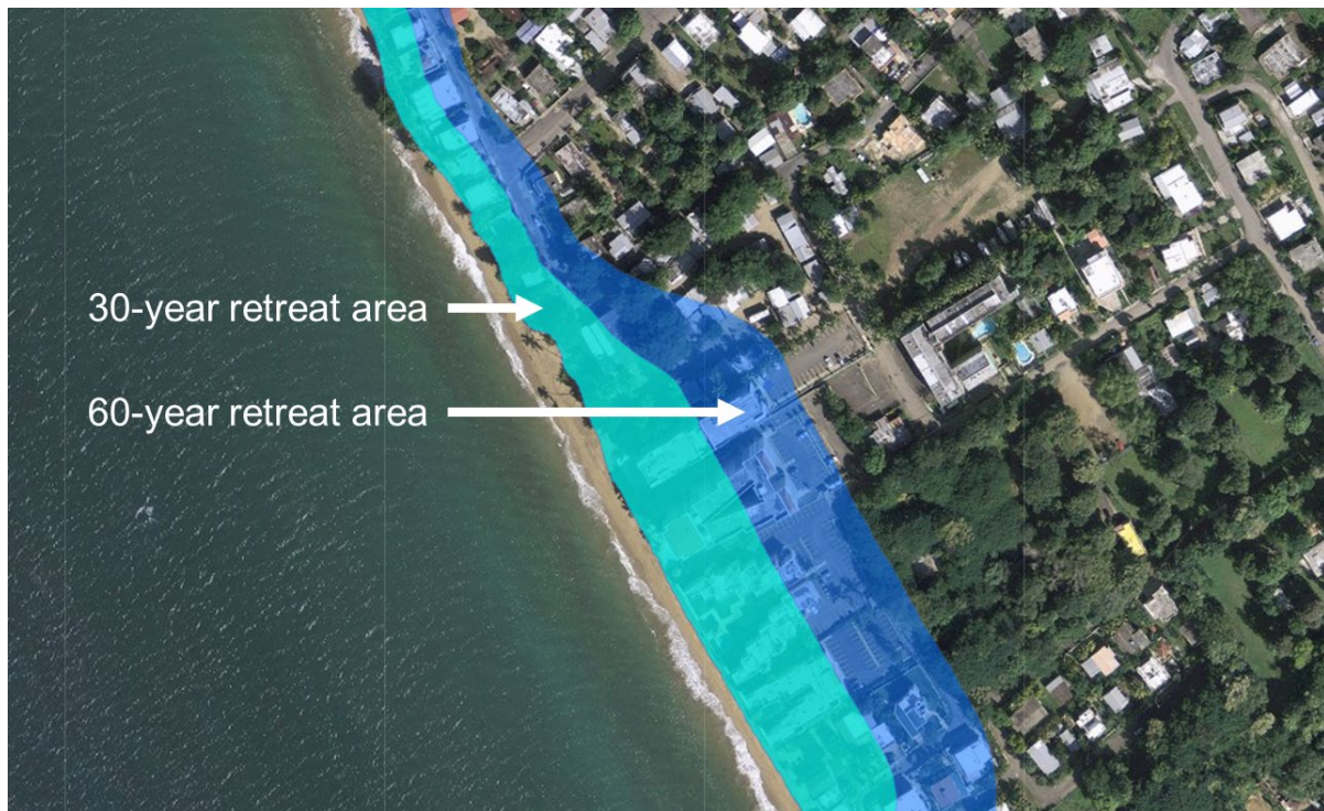
Figure 7: Example of future shoreline erosion areas created as an advisory product by FEMA to inform the resilient recover of Puerto Rico after Hurricane Maria.
