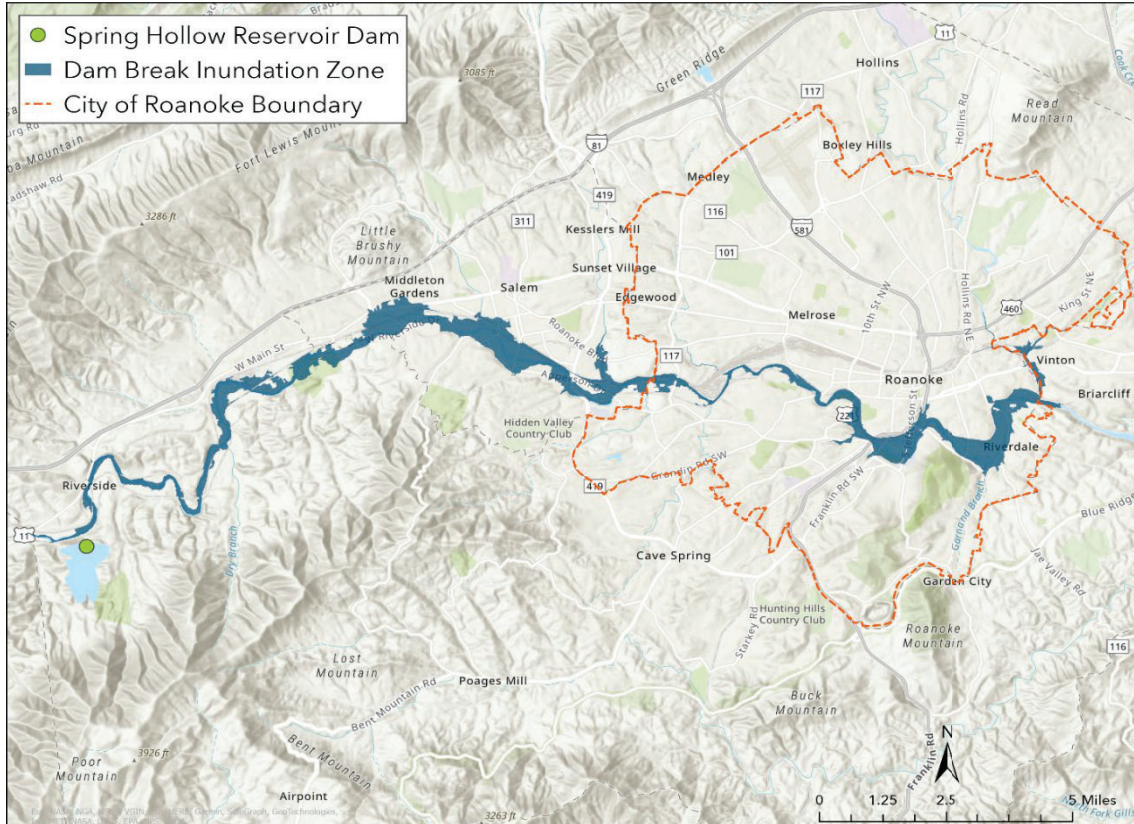
Figure 3 - The Spring Hollow Dam Break Inundation Zone and City of Roanoke Boundary. Zone boundary from the Virginia Department of Conservation and Recreation (DCR) Virginia Dam Safety and Inventory System (DSIS).
