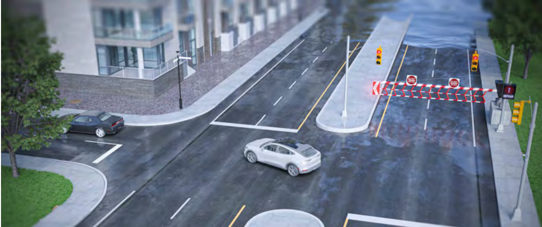
Flooded road gate system example (Source: Versilis)
